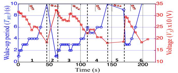
Figure 3: Adaptations of the wind-powered ED node. The node is powered on after a strong wind (interval 2 and 5) with a burst of harvested energy.
