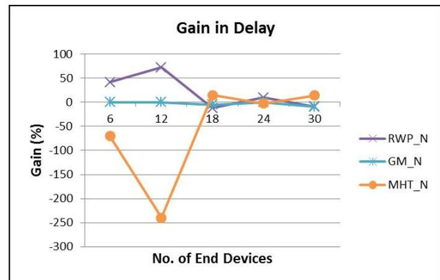
**Figure 8** Gain in delay of the probabilistic speculative algorithm in comparison with same-road algorithm
