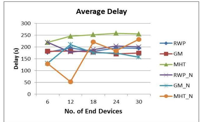
**Figure 4** Average delay during cell reselection procedures
