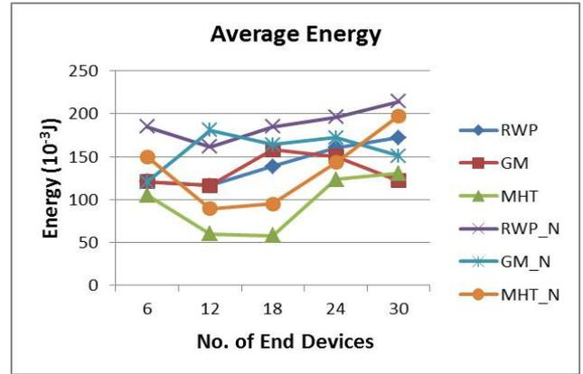
**Figure 3** Average energy during cell reselection procedures
