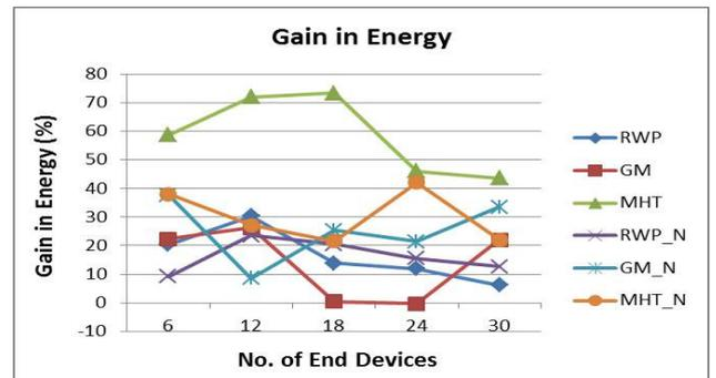
**Figure 5** Gain in average energy using 3 different mobility models
